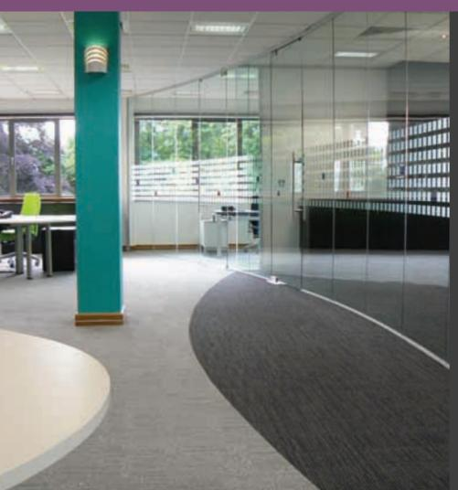
Available in either straight striking lines, faceted or the most graceful curves, Polar single glazed minimalist form is designed with the minimum of components, thus facilitating speed of erection without compromising structural stability and rigidity. The patented bubble joint ensures a virtually frameless system with no vertical posts between modules, corners or three way junctions.
