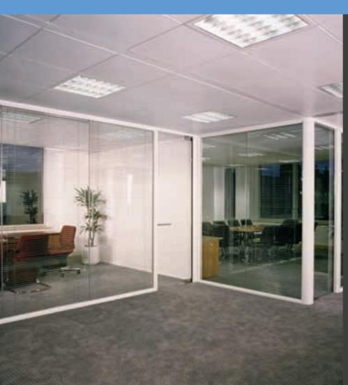
Komfire is a steel stud and plasterboard construction surrounded by an aluminium framework. This framework, together with the finishing trims, may be finished in any BS or RAL colour to complement each design.
